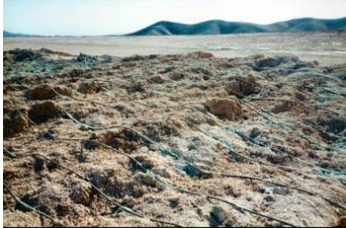
Figure 3. Detailed view of the irrigation system in a heap leach.
