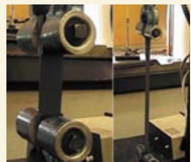
Photo 2: Exhumed PVC before and during tensile testing.
